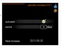
To prevent bacterial growth in the water heater, the heat pump can increase the hot water temperature for a short time at regular intervals.
