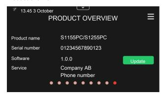
Here, you can find information about product name, the product's serial number, the version of the software and service. When there is new software to download, you can do it here (provided that S1155PC/S1255PC is connected to myUplink).
