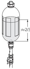
If the pressure in the system needs to be raised, this is done by closing the valve on the outgoing main line when the brine pump (GP2) is in operation and the level vessel (CM2) is open, so that liquid is drawn down from the vessel.
