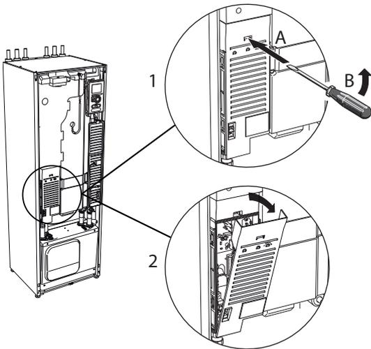
1. Insert the screwdriver (A) and pry the catch carefully downwards (B).
