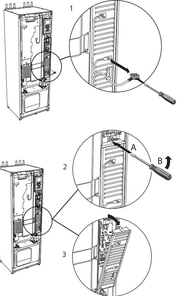
1. Disconnect the switches using a screwdriver.
