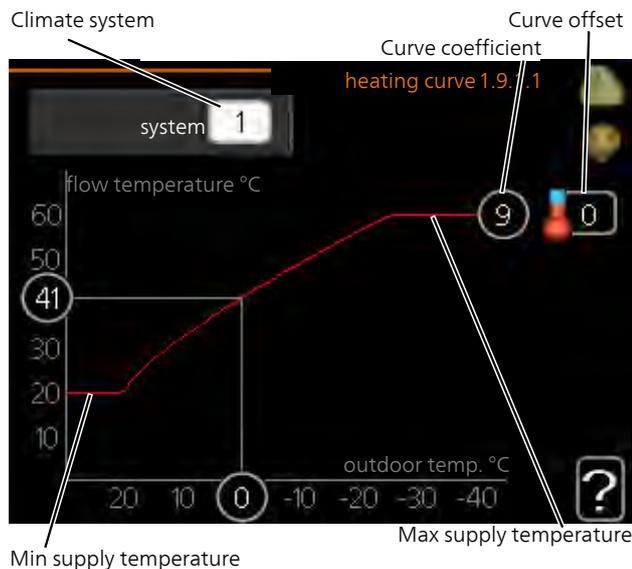
1. Select the climate system (if more than one) for which the curve is to be changed.
