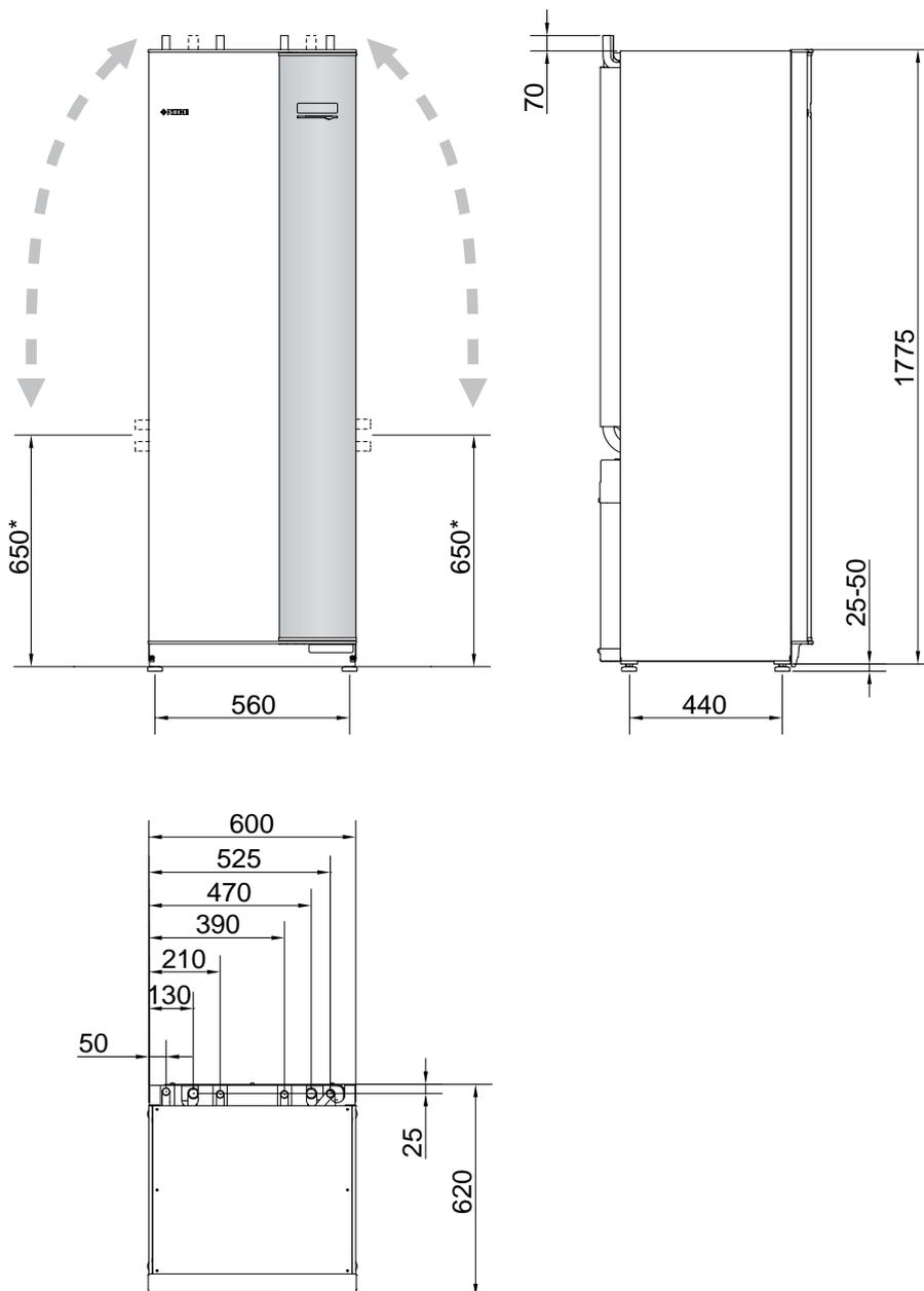
\* This dimension applies at 90° angle on the brine pipes (side connection). The dimension can vary approx. ±100 mm vertically as the brine pipes consist in part of flexible pipes.
