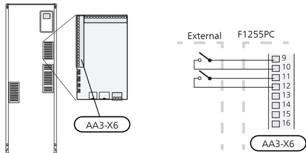
The example above uses the inputs AUX1 (X6:9-10) and AUX2 (X6:11-12) on the input board (AA3).
