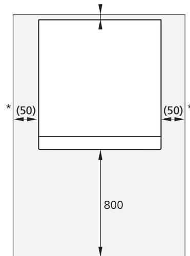
\* A normal installation needs 300 – 400 mm (any side) for connection equipment, valves and electrical equipment.
