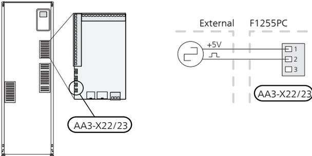
Activate the energy meter(s) in menu 5.2.4 and then set the desired value (energy per pulse) in menu 5.3.21.
