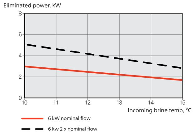
Passive cooling, 23 °C return temperature nominal flow brine/heating medium
