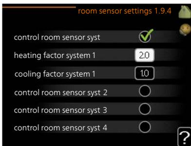
Room sensors to control the room temperature can be activated here.
