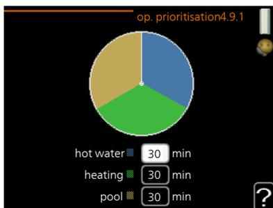
Choose here how long the heat pump should work with each requirement if there are two or more requirements at the same time. If there is only one requirement the heat pump only works with that requirement.
