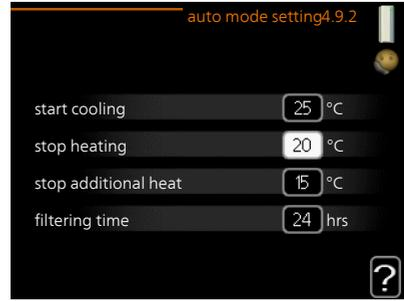
When the operating mode is set to "auto", the heat pump selects when start and stop of additional heat and heat production is permitted, dependent on the average outdoor temperature. You can also select start temperature for cooling.
