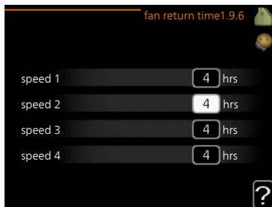
Here you select the return time for temporary speed change (speed 1-4) on the ventilation in menu 1.2.
