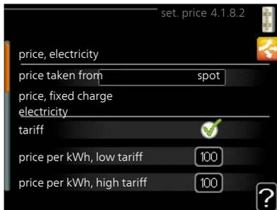
The function prioritises how / to what extent each docked energy source will be used. Here you can choose if the system is to use the energy source that is cheapest at the time. You can also choose if the system is to use the energy source that is most carbon neutral at the time.
