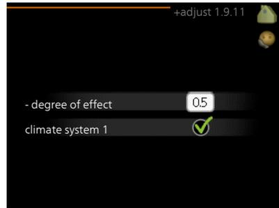
Using +Adjust, the installation communicates with the underfloor heating's control centre\* and adjusts the heating curve as well as the calculated supply temperature according to the underfloor heating system.
