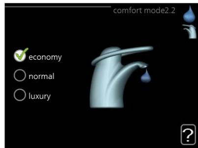
The difference between the selectable modes is the temperature of the hot tap water. Higher temperature means that the hot water lasts longer.
