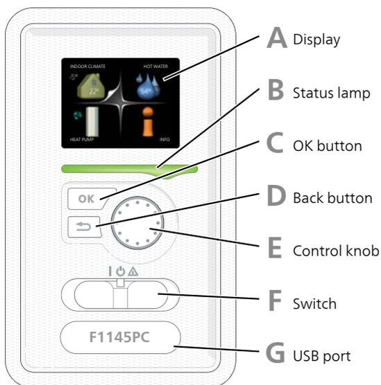
There is a display unit behind the heat pump door, which is used to communicate with F1145PC. Here you:
