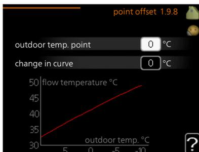
Select a change in the heating curve at a certain outdoor temperature here. One step is usually enough to change the room temperature by one degree, but in some cases several steps may be required.
