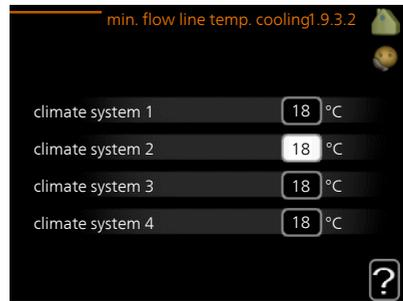
In menu 1.9.3 you select heating or cooling, in the next menu (min. supply temp.heating/cooling) set the minimum temperature on the supply temperature to the climate system. This means that F1145PC never calculates a temperature lower than that set here.
