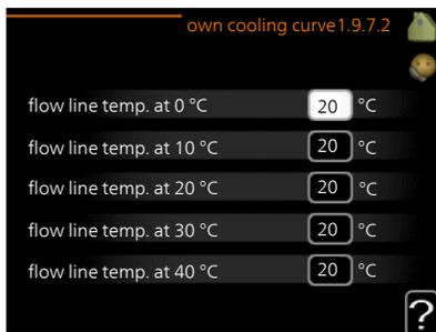
When required, create your own heating or cooling curve here, by setting the desired supply temperatures for different outdoor temperatures.
