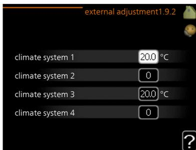
Connecting an external contact, for example, a room thermostat or a timer allows you to temporarily or periodically raise or lower the room temperature while heating. When the contact is on, the heating curve offset is changed by the number of steps selected in the menu. If a room sensor is installed and activated the desired room temperature (°C) is set.
