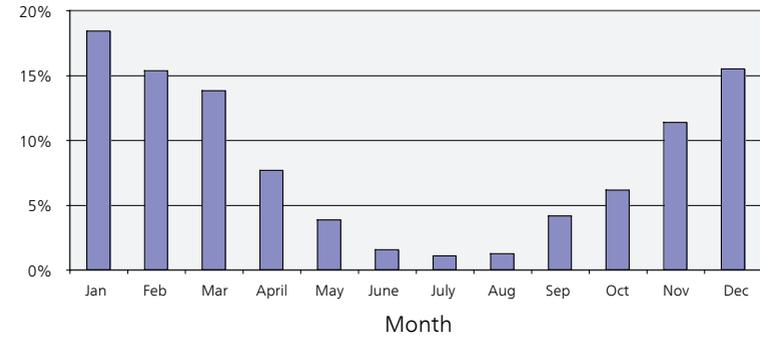
The diagram shows energy consumption during heating operation only. During cooling operation, the energy consumption can increase slightly during the hotter periods of the year.
