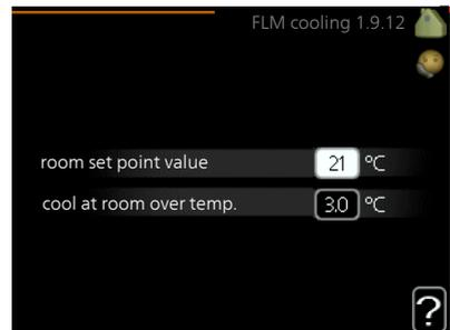
When you have activated FLM cooling in menu 5.3.1, set the desired room temperature in this menu. You also select at the temperature at which cooling is to start.
