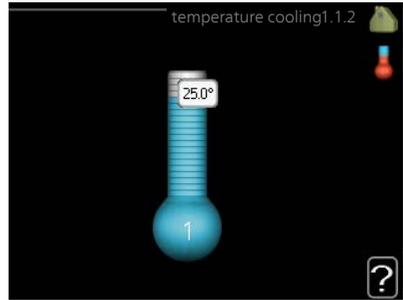
The value in the display appears as a temperature in °C if the climate system is controlled by a room sensor.
