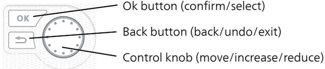
A detailed explanation of the button functions can be found on page 11. How to scroll through menus and make different settings is described on page 15.
