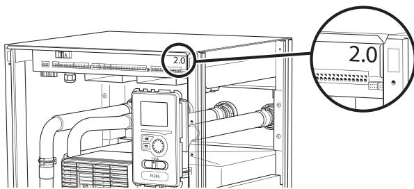
Use cable type LiYY, EKKX or similar with a cable area of at least 0,5 mm<sup>2</sup>.
