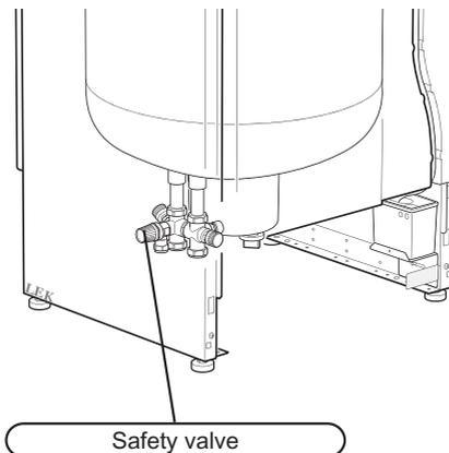
The safety valve must be checked about four times a year. The safety valve is reached by removing the main cover.
