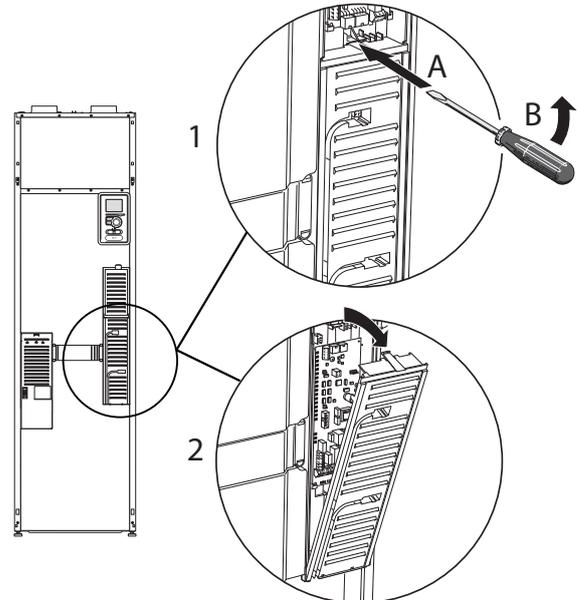
1. Insert the screwdriver (A) and pry the catch carefully downwards (B).
