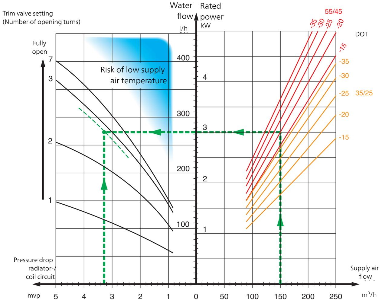
The delivered output in the diagram is calculated when dimensioning the heating system 55/45°C respective 35/25°C (underfloor heating).
