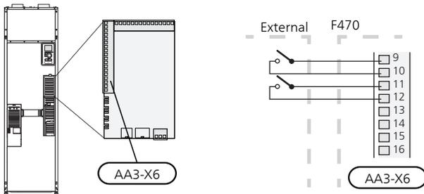
The example above uses the inputs AUX1 (X6:9-10) and AUX2 (X6:11-12) on the input board (AA3).
