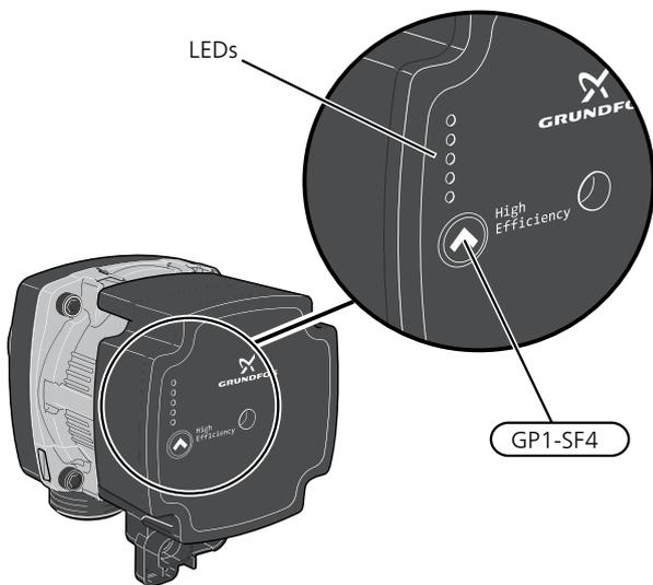
The circulation pump (GP1) is equipped with five LEDs. In normal mode, the LEDs show the power consumption. They can also indicate alarms or be used to display the pump speed.
