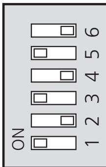
The image shows the dip-switch (AA1-S2) in the factory setting.
