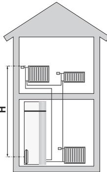
If the pre-pressure is not high enough, it can be increased by adding air via the valve in the expansion vessel. The expansion vessel's pre-pressure must be stated in the inspection document. Any change in the pre-pressure affects the ability of the expansion vessel to handle the expansion of the water.
