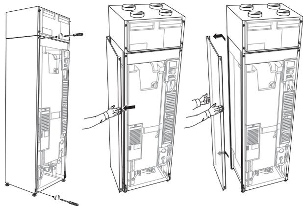
The side covers can be removed to facilitate the installation.
