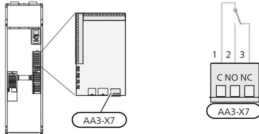
The picture shows the relay in the alarm position.
