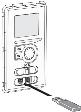
The display unit is equipped with a USB socket that can be used to update the software, save logged information and handle the settings in F470.
