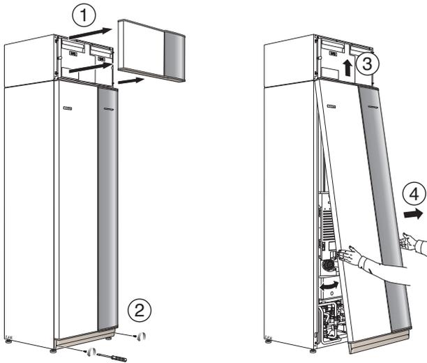
1. Remove the upper panel by pulling it straight out.
