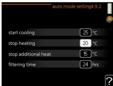
When the operating mode is set to "auto", the heat pump selects when start and stop of additional heat and heat production is permitted, dependent on the average outdoor temperature. You can also select start temperature for cooling.
