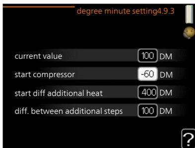
Degree minutes are a measurement of the current heating requirement in the house and determine when the compressor respectively additional heat will start/stop.
