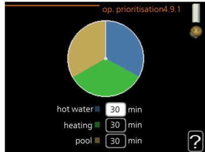
Choose here how long the heat pump should work with each requirement if there are two or more requirements at the same time. If there is only one requirement the heat pump only works with that requirement.
